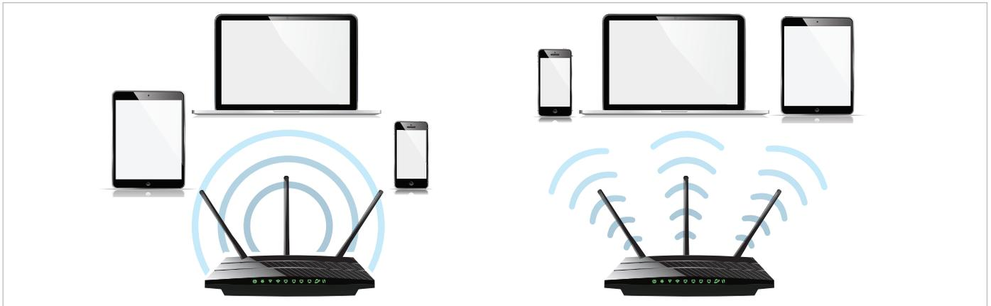
Figure 3. Example of beamforming with one spatial stream (left) and three spatial streams (right)<sup>3</sup>.
