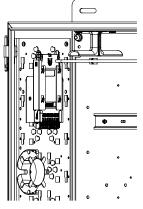
Step 4B: Enclosure Stack Bracket now attached to Enclosure Stack Base.
