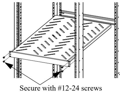
**Note:** Shelf is designed to support large networking equipment in combination with supplied equipment mounting flanges.
