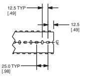
\*Adhesive tape is not meant for permanent mounting of wiring duct. One mounting hole on each end will be exposed for permanent mounting with fasteners. For best results, wiring duct should be applied to clean, dry, grease-free surfaces. We recommend the surface be cleaned prior to wiring duct installation.
