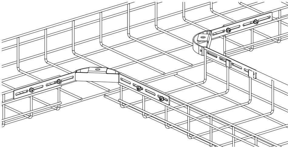
Assemble (1) radius support bracket to other side of basket. Keep supplied fasteners loose.
