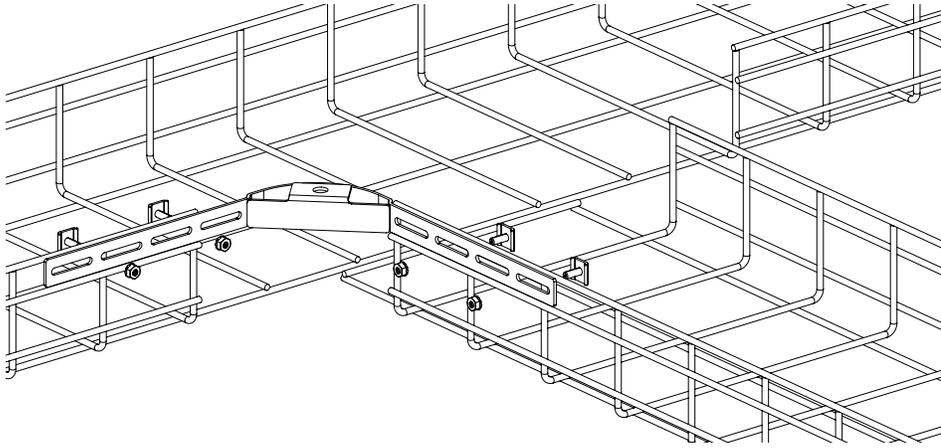
Assemble (1) radius support bracket to baskets. Keep supplied fasteners loose.
