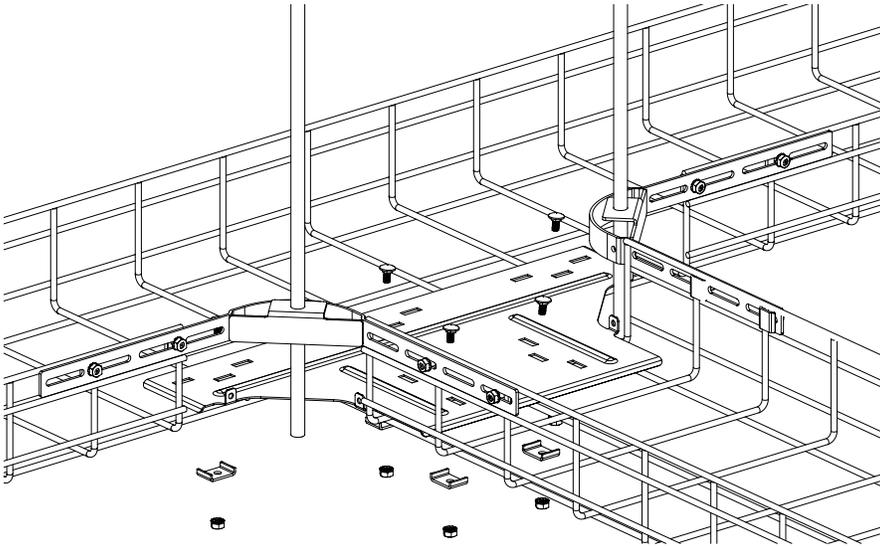
Add (1) connection plate to cover the gap between the baskets. Loosely attach with supplied fasteners.
