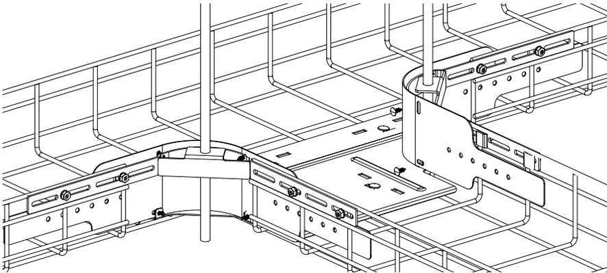
Place the (2) protective sheets along the radius of the corner. Attach with push-in fasteners and cable ties if desired.
