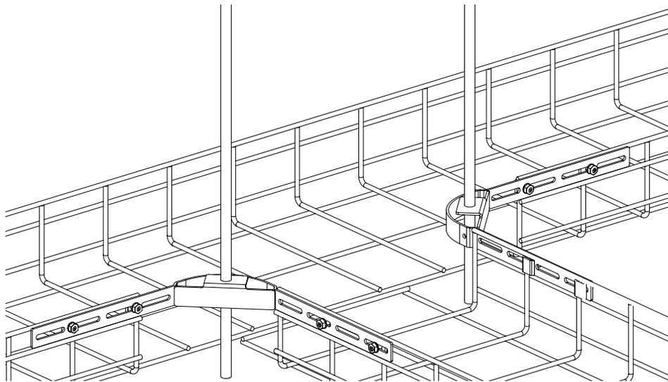
Hang basket. Assemble to customer supplied threaded rods. All trapeze brackets to be within 2 feet from intersection.
