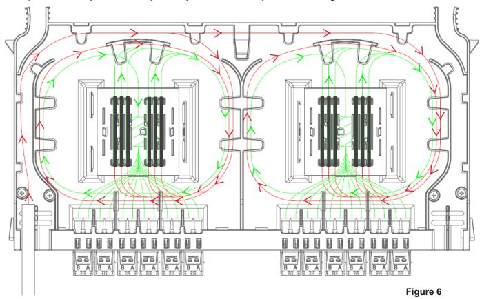
Discrete Splice. Cable Input to LC Adapter Output - Right Hand Input Wire Routing
