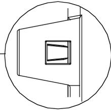
Ensure end cap and coupler(s) connect to junction box cover as shown [8 places]
