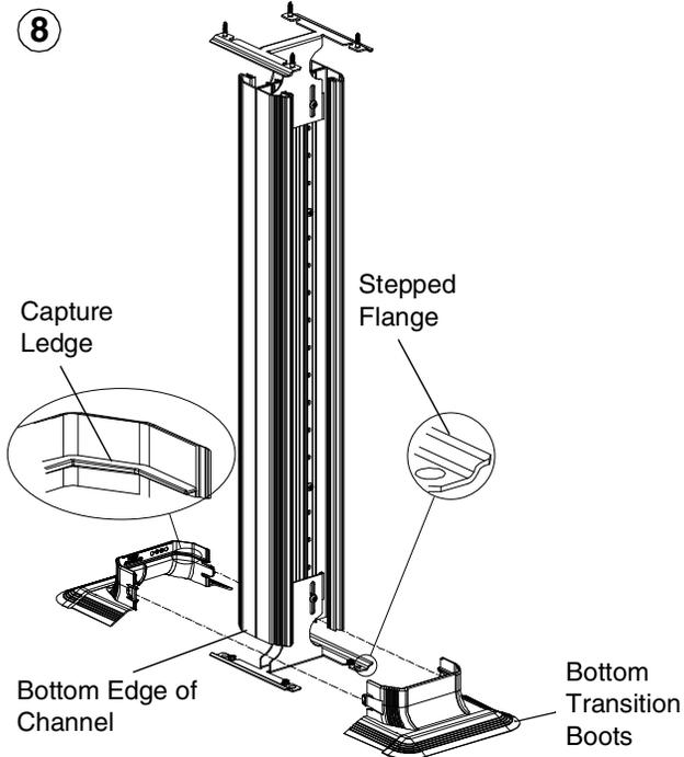
Assemble bottom transition boots together. Transition boot latches (shown in step 7) will mount to stepped flanges of the mounting brackets. Place bottom of channel on top of capture ledge of transition boots.
