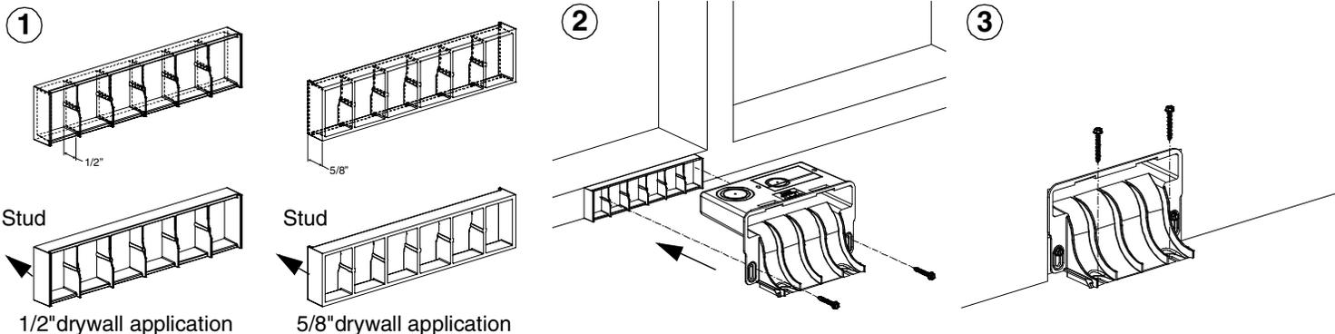
Determine if you will use 1/2" or 5/8" drywall. Orient standoff as shown for desired application.
