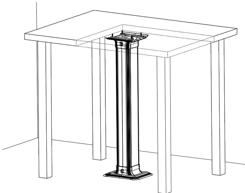
**NOTE:** Desired hole in table should be offset from table leg center to accommodate proper mounting of table leg.
