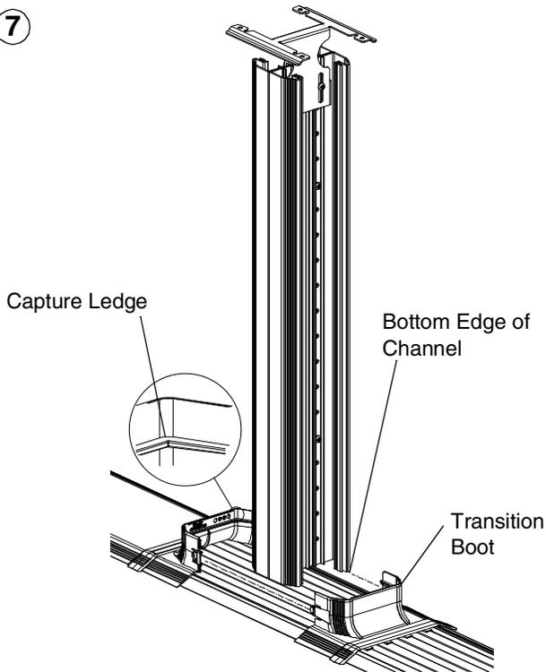
Set bottom edge of channel on capture ledge of installed transition boot. Connect second transition boot to the first.
