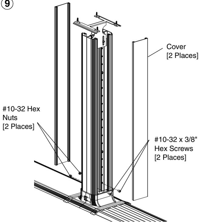
Route cables prior to installing covers. Covers are tamper-proof and are not intended for easy removal.
