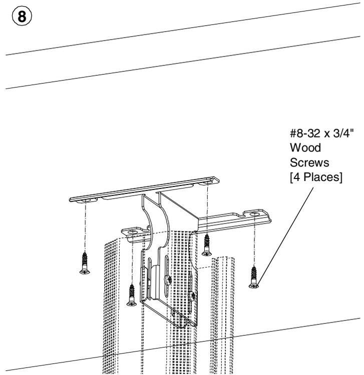
Ensure channel is level. Secure mounting bracket to underside of table using provided hardware. Fully tighten mounting bracket screws to secure channel in place.
