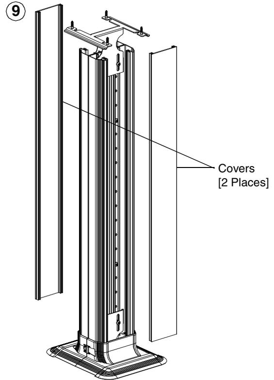
Route cables prior to installing covers. Covers are tamper proof and are not intended for easy removal.
