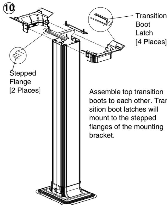
Assemble top transition boots to each other. Transition boot latches will mount to the stepped flanges of the mounting bracket.
