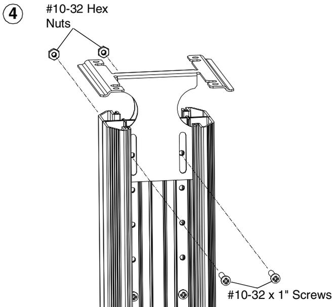
Secure mounting brackets to top and bottom of channel using provided hardware. Use the holes closest to the ends of the channel for assembly. Do not fully tighten the mounting bracket at this time.
