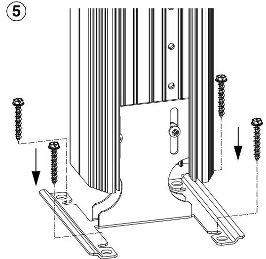
Pre-drill holes in infrastructure if necessary. Secure bottom mounting bracket to floor with proper hardware. (Concrete screws provided)
