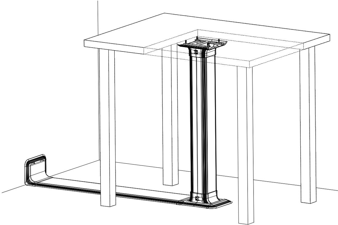
**NOTE:** For single side raceway application; above floor raceway should be mounted prior to table leg installation. Center of table leg will sit approximately 3-1/4" from the edge of the raceway cover. Route cables prior to installing the raceway cover.
