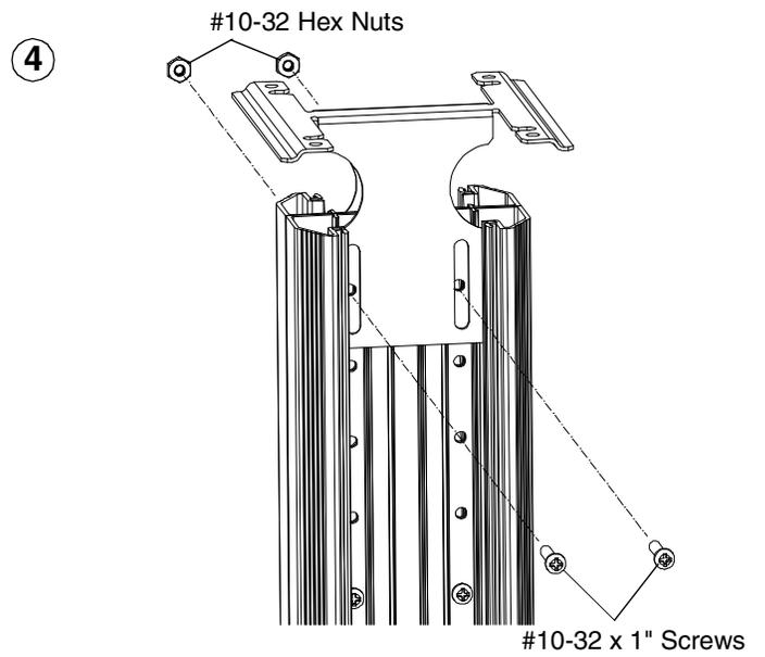
Secure mounting bracket to top of channel using provided hardware. Use the top hole of the channel for assembly. Do not fully tighten the mounting bracket at this time.
