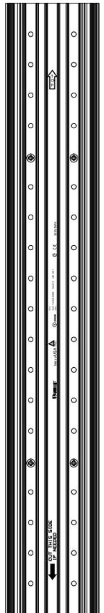
Measure the height from the floor to the underside of the table. Channel should be between 3-1/2" to 4" shorter than the measured height. If necessary, cut channel from bottom edge to accommodate.
