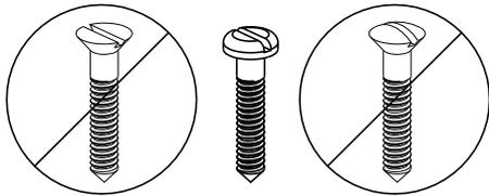
The mounting hardware used to secure the raceway shall be appropriate for the mounting surface.
