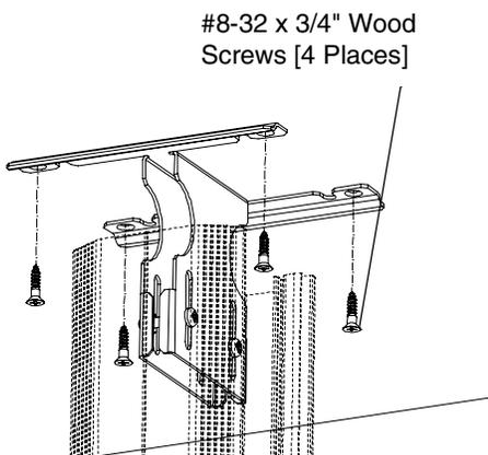
Ensure channel is level. Secure top mounting bracket to underside of table using provided hardware.
