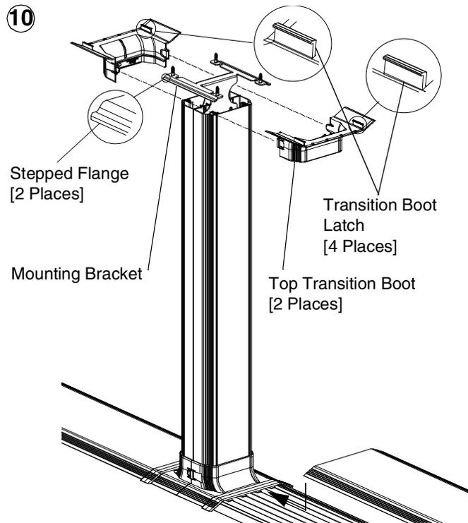
Assemble top transition boots to each other. Transition boot latches will mount to the stepped flanges of the mounting bracket.
