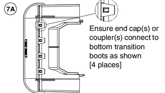
Ensure end cap(s) or coupler(s) connect to bottom transition boots as shown [4 places]
