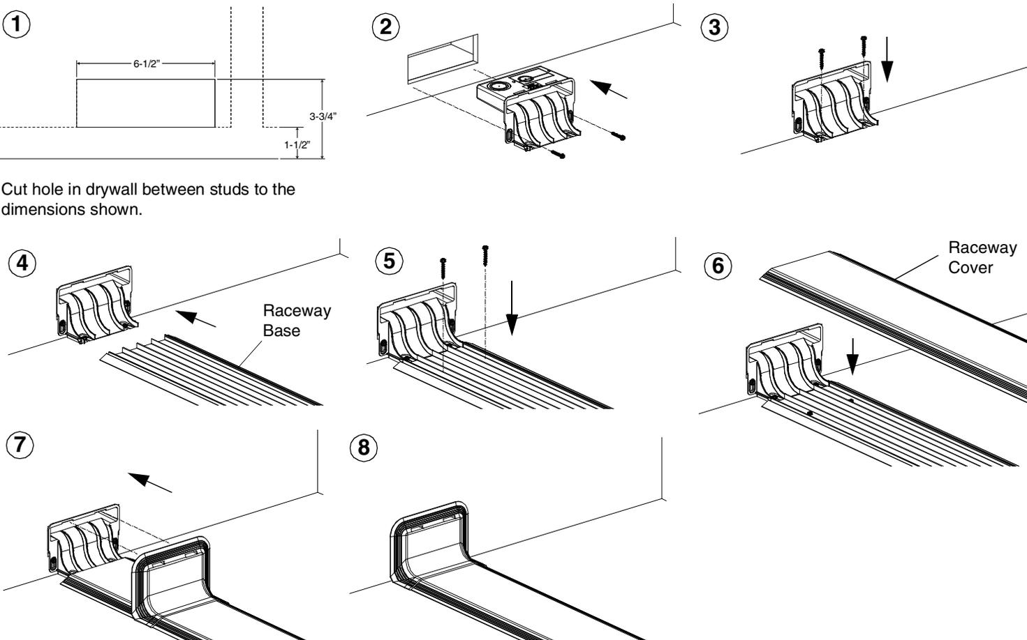
Cut hole in drywall between studs to the dimensions shown.
