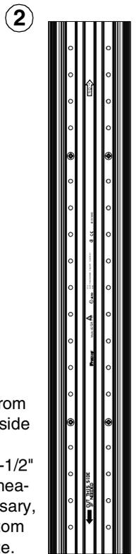
Measure the height from the floor to the underside of the table. Channel should be between 3-1/2" and 4" shorter than measured height. If necessary, cut channel from bottom edge to accommodate.
