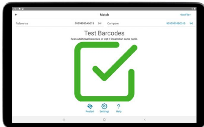
The mobile app **matches** the opposite end of a scanned cable. The software offers notifications when the right end is found, which expedites a tedious process to free up network engineers for more rewarding initiatives.
