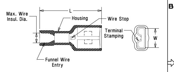
STRONGHOLD FEMALE DISCONNECT (250 SERIES) FULLY INSULATED NYLON, #12-10 AWG
