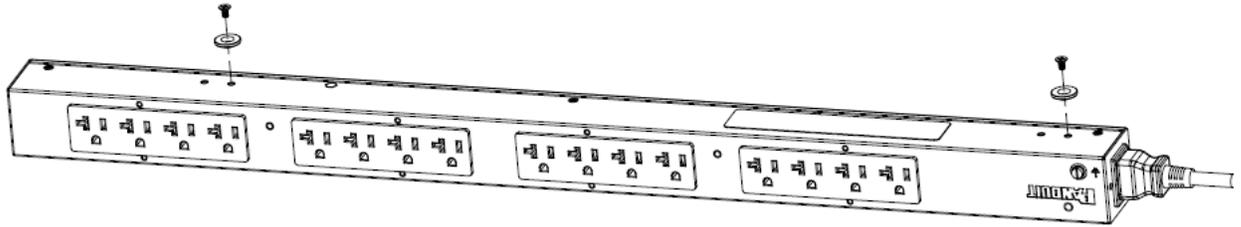
2. Install the PDU by inserting the mounting buttons into the keyhole slots on the PDU mounting bracket in the rack.
