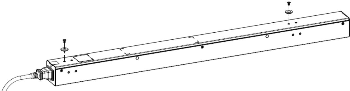
2. Install the PDU by inserting the mounting buttons into the keyhole slots on the PDU mounting bracket in the rack.
