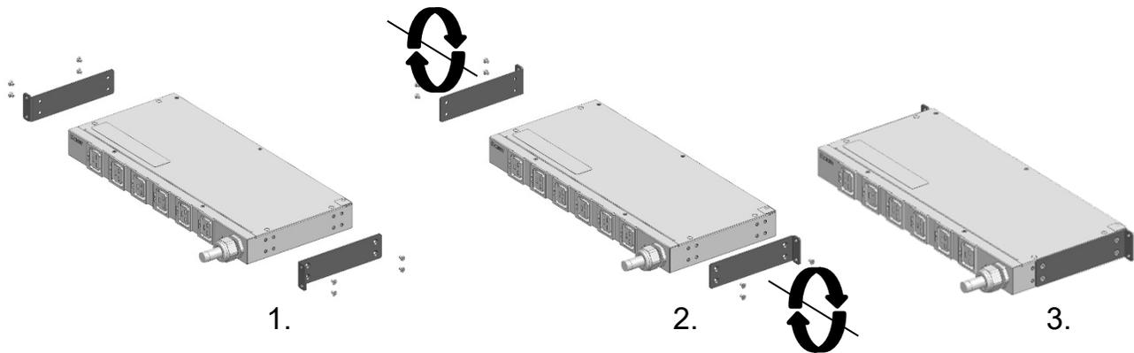
1. Remove the 4 screws holding each ear on.
