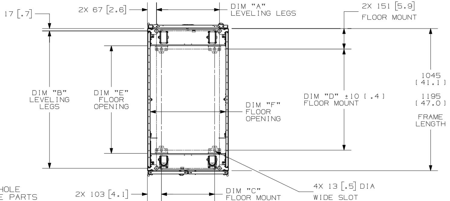
FLOOR MOUNTING HOLE LOCATIONS - SOME PARTS REMOVED FOR CLARITY
