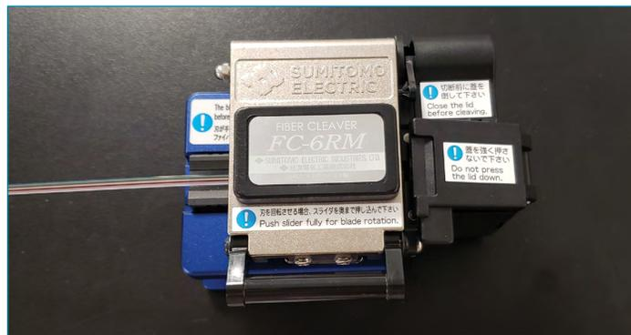
Figure 9: Cleaving the bare fiber(s).
