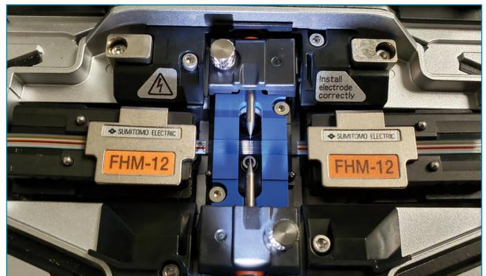
Figure 14: Image of completed arc process, fibers fused.
