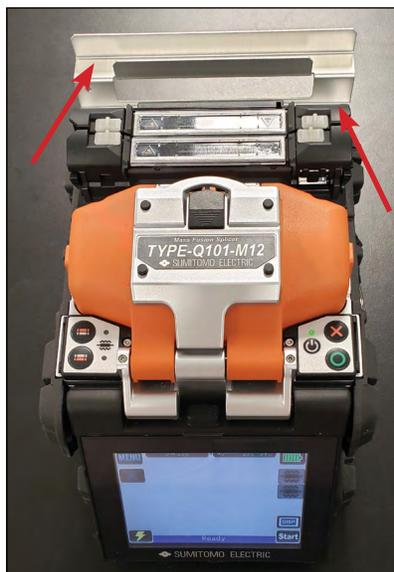
**Figure 18:** View of dual cooling trays.
