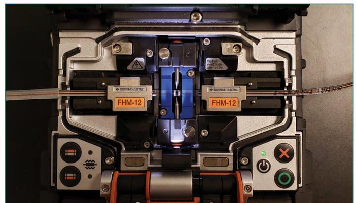
Figure 11: Bare fiber sections loaded into Splicer.
