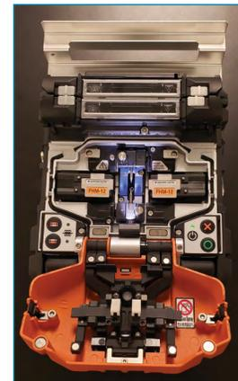
**Figure 4:** Fusion Splicer shown open, Fiber Sheaths closed.
