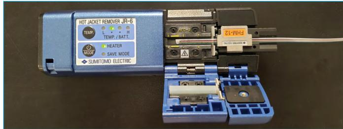
Figure 7: Removing the jacket from the fiber.
