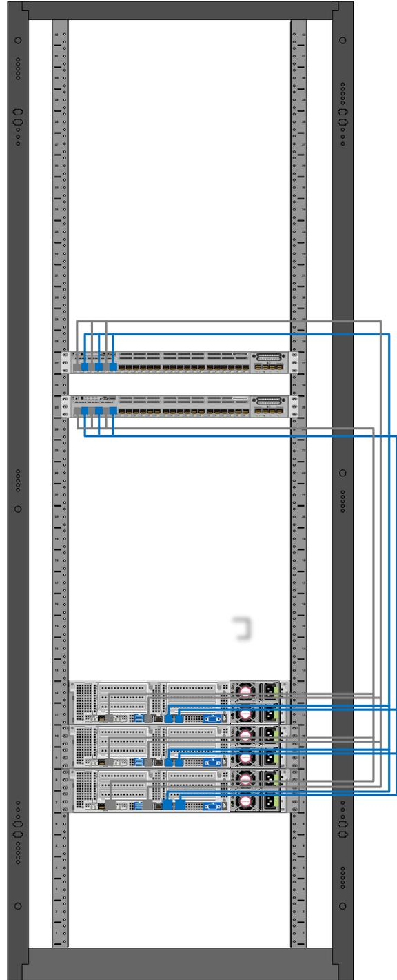
Figure 1 Basic copper connectivity
