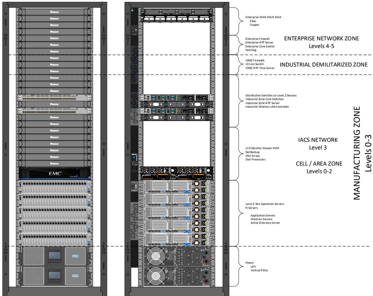
Figure 5 Planning the Elevation in the 42 RU NEMA 12 MDC
