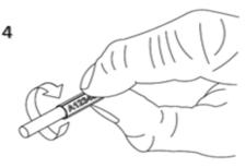
Once the label is completely applied to the cable, pinch lightly and rotate it in the same direction as you wrapped it. This will break the label perforation and separate the label from the anchor.
