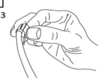
Wrap the label around the cable and over upon itself until completely wrapped.
