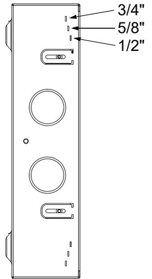
Line up edge of stud with proper drywall thickness slot.
