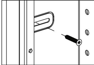
Stud spacing must be 16" on center for proper installation.
