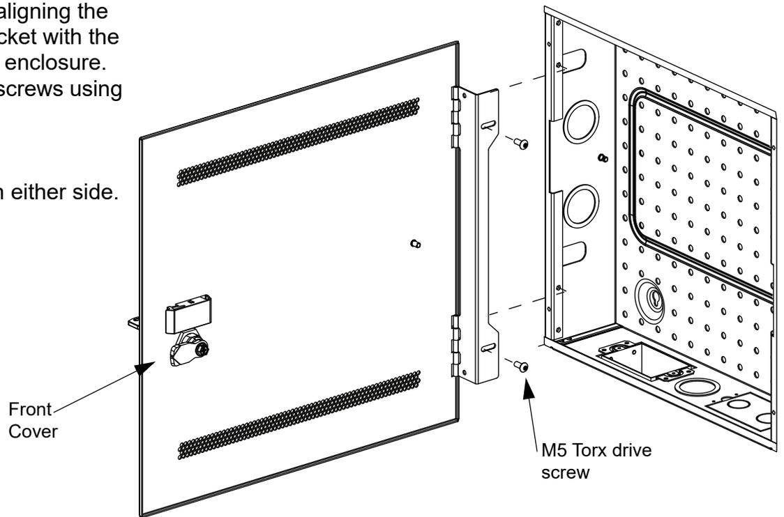
1. Install door latch plate by aligning the slots of the cover bracket with the threaded holes of the enclosure.
