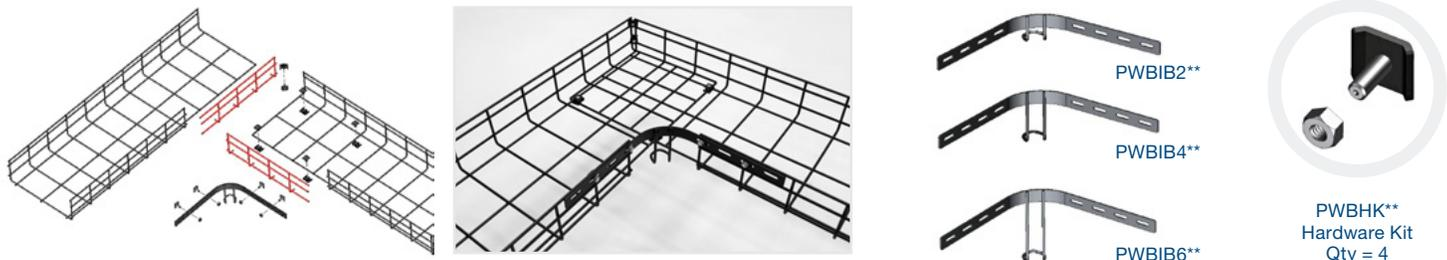
1. Cut away large section of sidewall at end of each of the two pathways (Reference table to the right)
