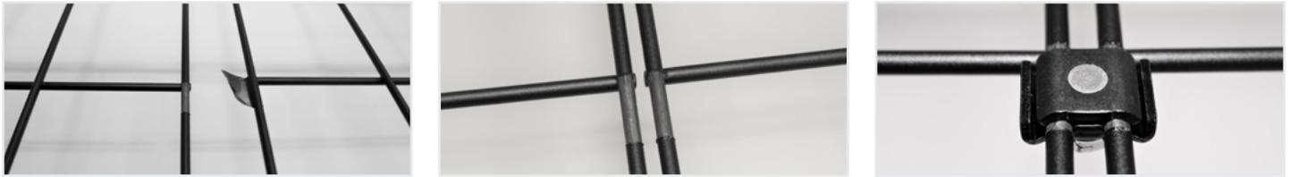
PWBSPLBL and PWBSPLEZ Bolt on Splices provide a UL Classified bond when installed on areas where the paint has been removed. Powder coated baskets include a masking tape feature that can be removed to expose bare metal on each end. If the the basket is cut, the user should remove the paint from the metal, if it is not an electro zinc version.
