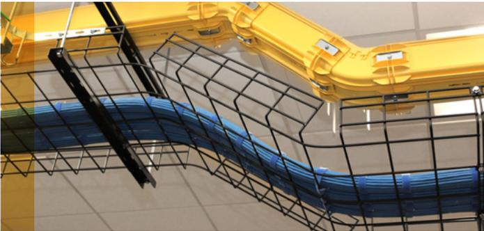
Vertical level changes are easily formed by cutting away sidewall sections on each side of the basket and bending the pathway to the desired angle.
