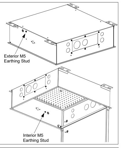
MSGK door bonding kit (sold separately) includes one quick-disconnect jumper to bond the door to the enclosure. Attach each end of the bonding jumper to the specified M5 bonding studs using the bonding nuts provided with the MSGK kit.
