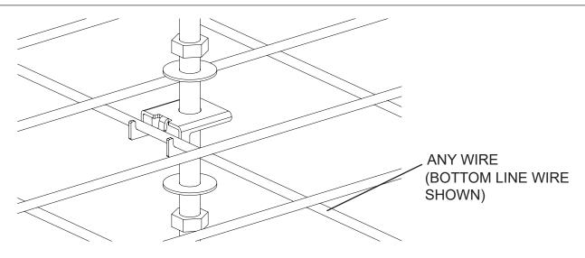
USE ONLY 1/2" OR 12MM THREADED ROD WITH THE TRAPEZE SUPPORT BRACKET.
