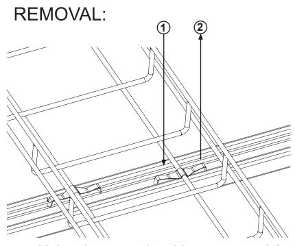
PRESS ON 1 SIDE AND USE A SCREWDRIVER TO SWITCH STRUT CLIP OFF,
