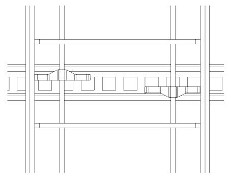
THE SECOND CLIP IS INSTALLED ORIENTATED FACING THE OPPOSITE WAY AS SHOWN.
