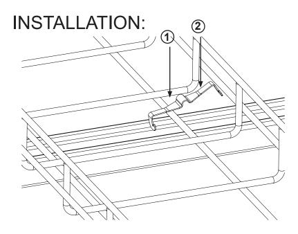
USE FINGER TO PUT ONE SIDE IN FIRST AND PRESS THE OTHER SIDE DOWN AND ROTATE INTO PLACE.
