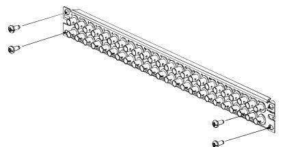
2. Align screws with desired holes on rack.
