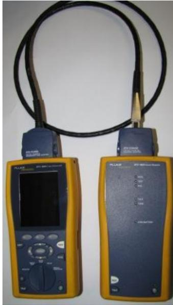
For detailed instructions on Set Reference procedure, refer to Fluke Network's *DTX-1800 Series Users Manual* page 20, on "Setting the Reference for Twisted Pair Cabling". The link for the User's Manual is:
