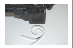
Remove the wound up excess tie length piece.
