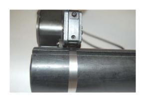
Actuate Tension Handle by squeezing the Tension Handle and Upper Handle together.
