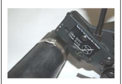
Holding the handles together, grasp the Cutter Handle Lever and move it forward. This action will set ball and cut off the excess tie length flush with the tie head.
