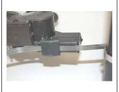
Insert the end of the tie into the tool between Setshear Finger (#1) and Anvil (#2).
