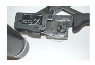
As the tie end is fed through the tool insert the tie end through the Tensioning Split Mandrel. Pull tool tight to bundle.
