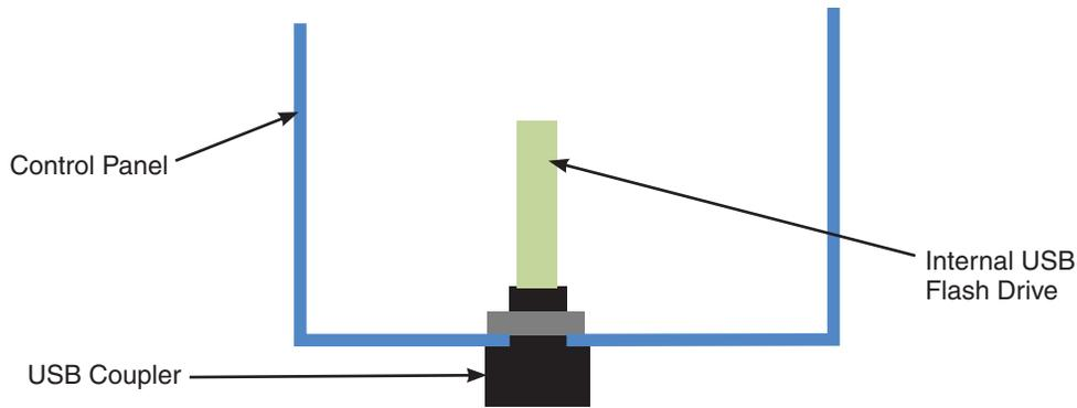
**Figure 5: Use Case Showing Internal USB Drive**
