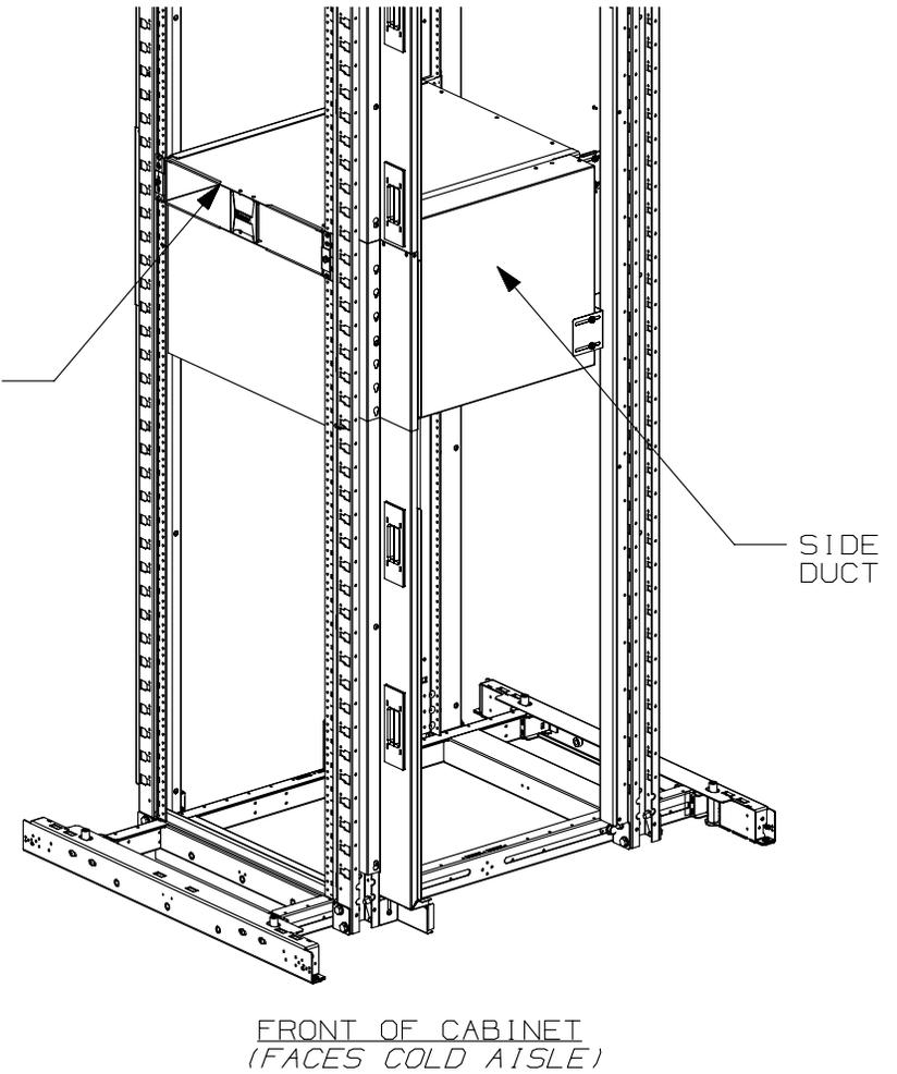
1. VERTICAL BLANKING PANELS MUST BE USED WITH THIS PRODUCT TO PREVENT EXHAUST RECIRCULATION.
