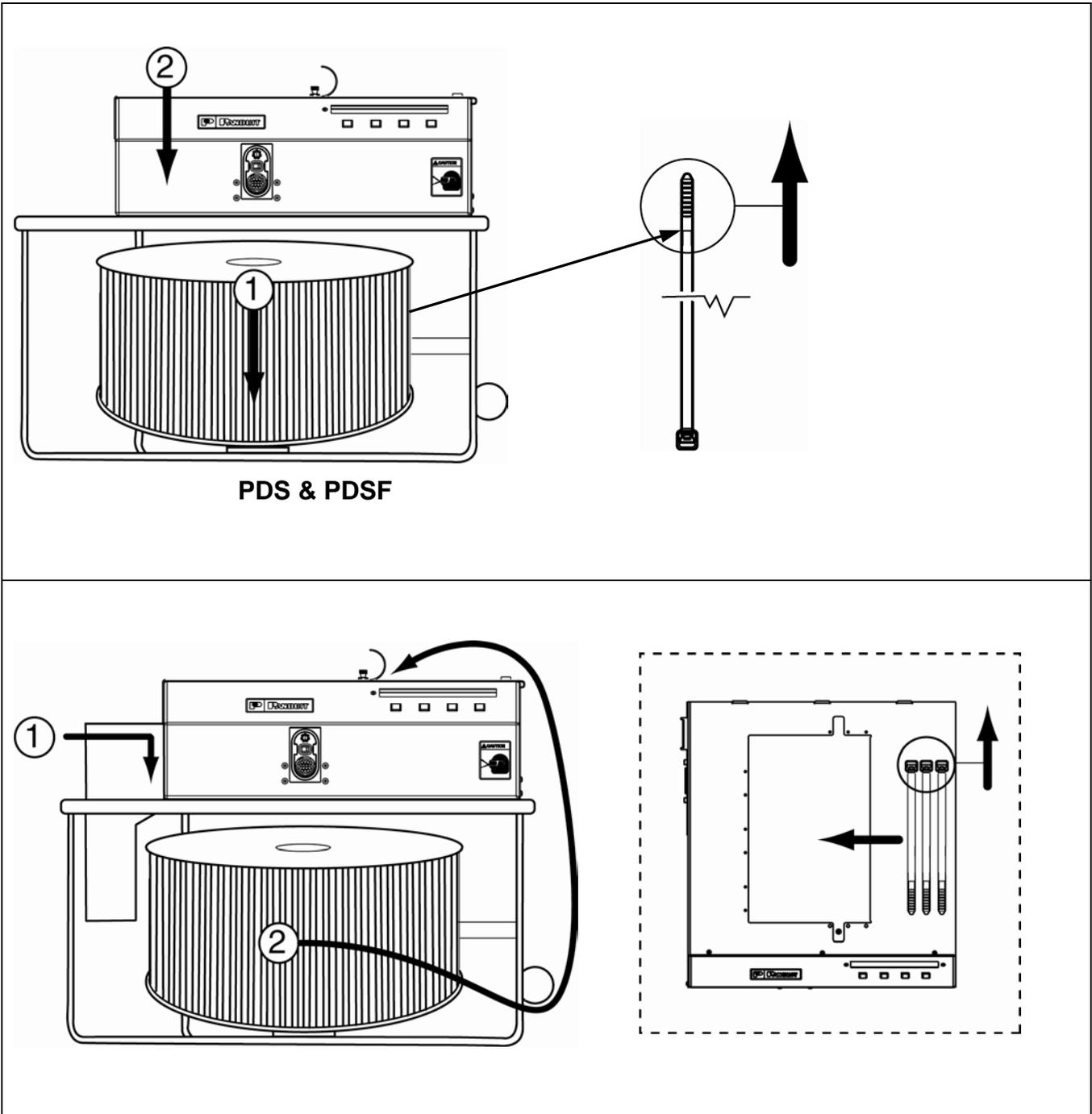
Always position the dispenser and frame in the work area so there are no severe bends or twists in the PHS Feeder Hose.
