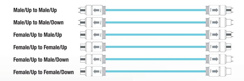
Achieve the most accurate link test measurements with any test equipment. Whether test equipment has a male or female interface, the PanMPO™ Connector can be configured to fit, without introducing a third test cord. This eliminates an added layer of variability, reduces errors and improves accuracy.
