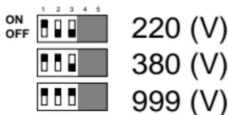
VT connection: set dip-switches 1, 2 and 3 according to what is shown in the figure on the left. The 100VAC input can be connected to a VT with a secondary of 100VAC and a primary of 220V, 380V or 1000V; the relating primary selection must be done as indicated on the left.
