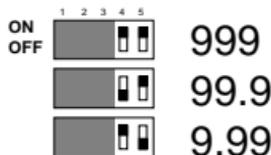
Remove the front cover of DI3-DIN as indicated in figures 9 and 10. For the decimal point selection, use dip-switches 4 and 5 as shown in the figure on the left.
