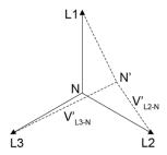
$$\begin{split} & V_{\text{ANOM}} = V_{\text{L1-N}} = V_{\text{L2-N}} = V_{\text{L3-N}} \\ & \text{max } |\Delta V_{\text{PH-N}}| = |V'_{\text{L3-N}} - V'_{\text{L2-N}}| \\ & \text{max } |\Delta V_{\text{PH-N}}| = 0 \Rightarrow \text{ASY} = 0 \end{split}$$
