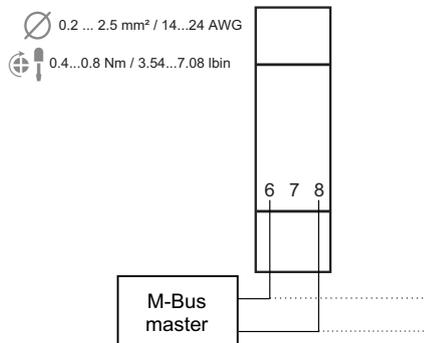
**Fig. 7** M-Bus
