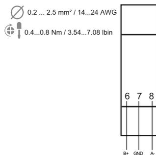
**Fig. 8** Port RS485
