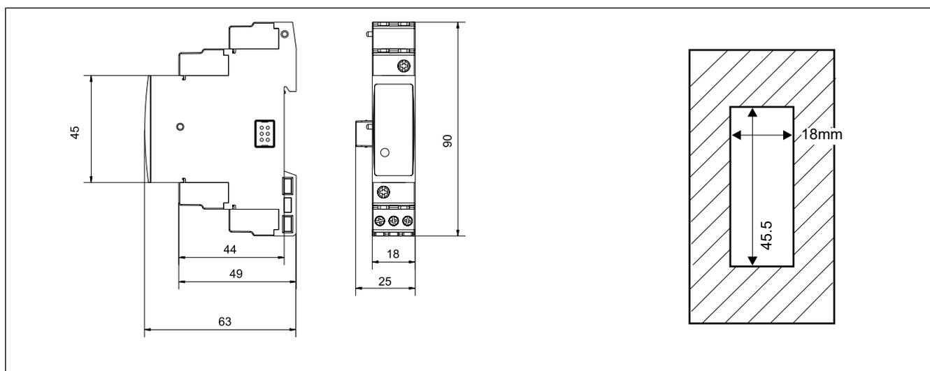
**VMU-1 Dimensions and panel cut-out (mm)**
