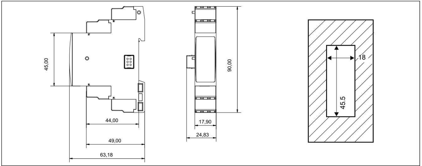
**VMU-P Dimensions and panel cut-out (mm)**
