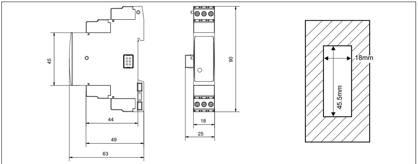
**VMU-O Dimensions and panel cut-out (mm)**
