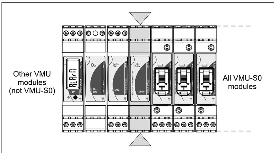
The VMU-1 has to be mounted between the group of VMU-S0 and all the other modules as shown in the example picture on the left.
