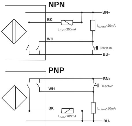
**By means of the Teach-in wire, the functions described in the Teach-in Guide can be set up.**
