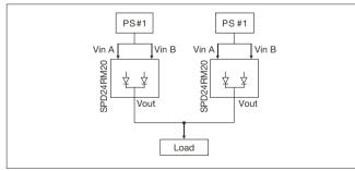
3.) 1+N Redundancy: Using more than one PS as redundant units to increase the reliability.
