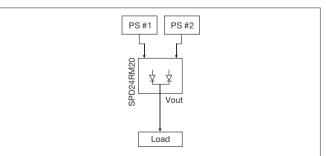
2.) Single Use: Connecting only one PS to one SPD24RM20 to reduce the stress of the diodes and hence increase the reliability.
