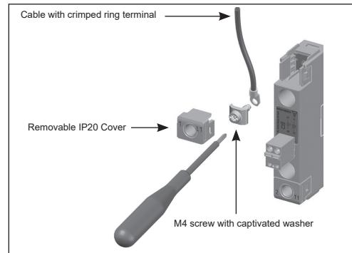
**Terminations | Termineringer | Terminales | Anchlässe | Terminations | Terminali | Клеммы | 端接**
