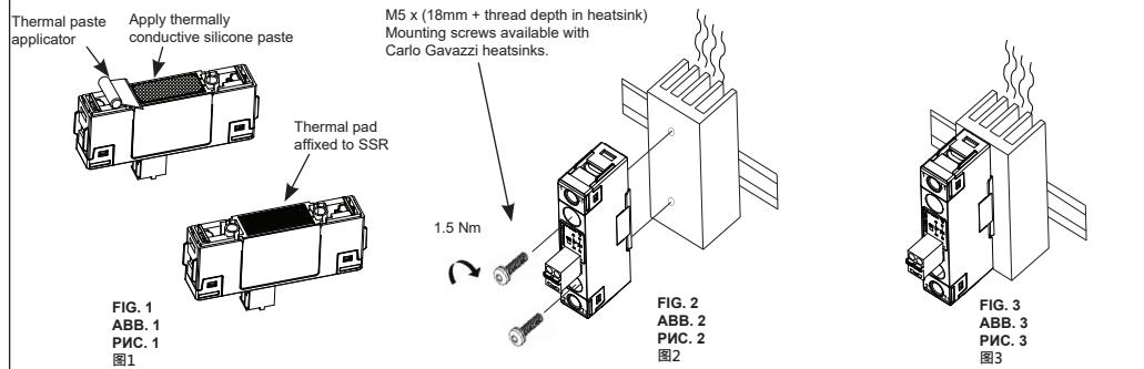
**FIG. 1:** A thin layer of thermally conductive silicone paste must be evenly applied to the base of the SSR. In case of a thermal pad attached to the base of the SSR, no thermal paste is required.
