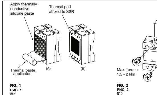
**FIG. 1:** A thermal interface is required between SSR and mounting surface. Thermally conductive silicone paste shall be applied and spread throughout the base of the SSR (A). Alternatively, an interface material with adhesive on one side shall be affixed to the baseplate of the SSR before mounting the SSR on the heatsink (B).
