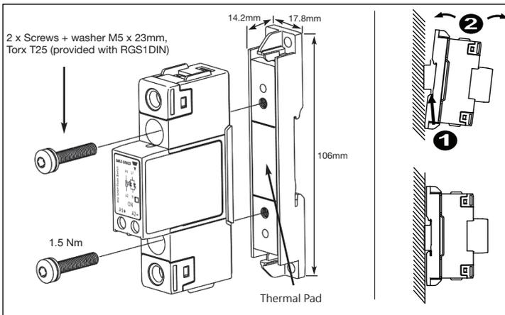
**Terminations | Termineringer | Terminales | Anschlüsse | Terminations | Terminali | Клеммы | 端接**
