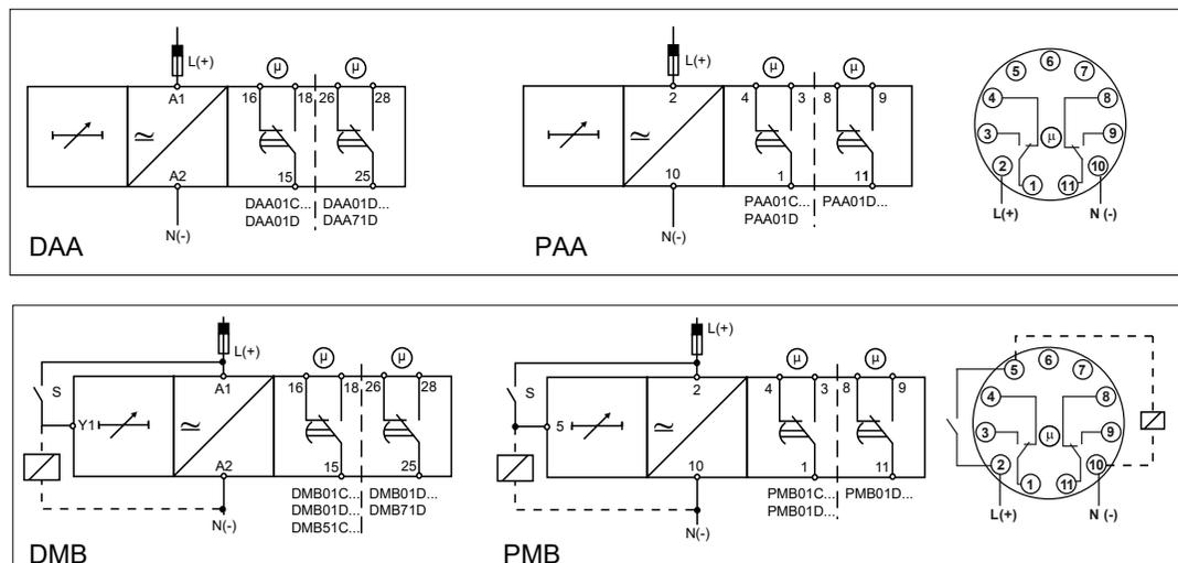
Connect the power supply to the proper terminals. Connect the trigger input S between terminals A1 and Y1 (DBA52 and DMBX1 versions only). Connect the relay output according to the ratings as shown in the side diagrams.
