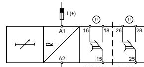
Connecting pins + and A2 it's possible to test the non-replaceable built-in Ni-MH battery charge value (DBB02 only).
