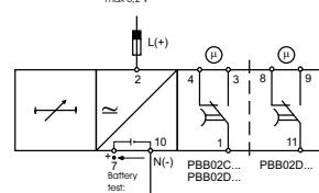
Connecting pins 7 and 10 it's possible to test the built-in non-replaceable Ni-MH battery charge value (PBB02 only).
