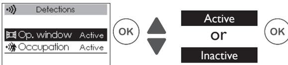
If devices are connected together, you can disable Open window detection on a single device without disabling the other (see "Settings" in the "Expert Menu").
