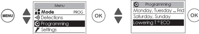
Regulates the temperature reduction level you want outside of comfort ranges (from  $-2^{\circ}\text{C}$  to  $-9^{\circ}\text{C}$ ). By default, it is set at  $-3.5^{\circ}\text{C}$  (if the set temperature is  $19^{\circ}\text{C}$ , as a result, outside of Comfort ranges, it will fall to  $15.5^{\circ}\text{C}$ ).
