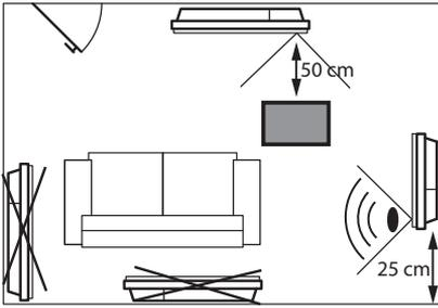
To optimize the absence detection of your device, avoid installing it in a closed corner or behind a piece of furniture.
