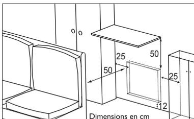
Comply with the minimum distances from any furniture units when positioning the device.
