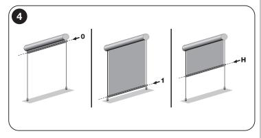
When the limit switches are not programmed yet, the roller shutter can be moved only in the "hold-to-run" mode, i.e. keeping the control key pressed for the desired duration of the manoeuvre; the movement stops as soon as the user releases the key. However, after programming the limit switches, briefly pressing the appropriate key will start the roller shutter and it will stop moving automatically as soon as the roller shutter reaches the required position.
