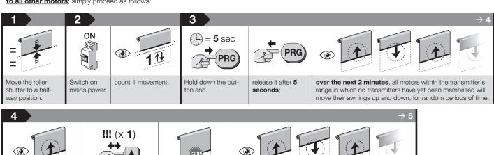
Select the roller shutter you wish to program and, at the start of an UP movement, stop it IMMEDIATE-LY, by pressing and releasing the button (1 time):
