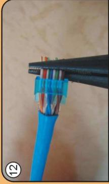
12 To pull the conductors lean gently against the fulcrum by pliers until the manage tool flush with H Divider
