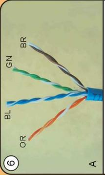
6 To put H\_divider into the conductors (blue pair and green pair are in opposite direction)
