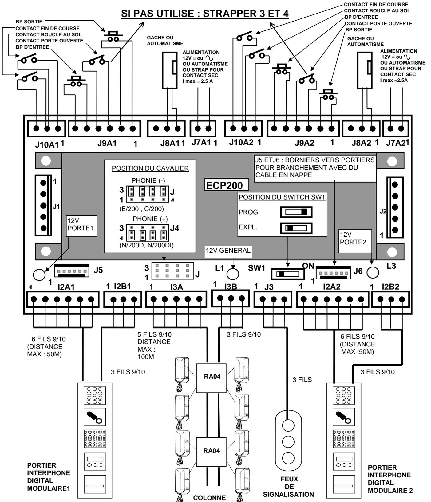
**RACCORDEMENT CENTRALE ECP200+RECEPTEUR D'APPEL RA04
