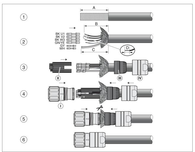
Figure 14: Assembling motor cables with M40 motor connector
