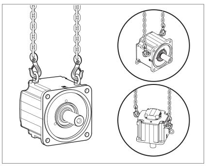
*Mounting* When the motor is mounted to the mounting surface, it must be accurately aligned axially and radially and make even contact with the mounting surface. All mounting screws must be tightened with the specified tightening torque. No uneven mechanical load must be applied when the mounting screws are tightened. See chapter "2 Technical Data" for data, dimensions and degrees of protection (IP).
