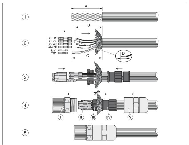
Figure 13: Assembling motor cables with M23 motor connector
