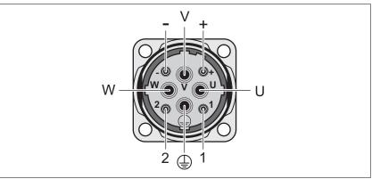
Figure 10: Pin assignment motor connection M40
