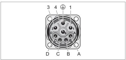
Figure 9: Pin assignment motor connection M23
