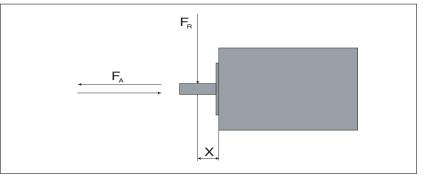
Figure 6: Shaft load
