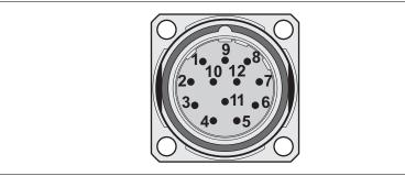
Figure 11: Pin assignment encoder connector
