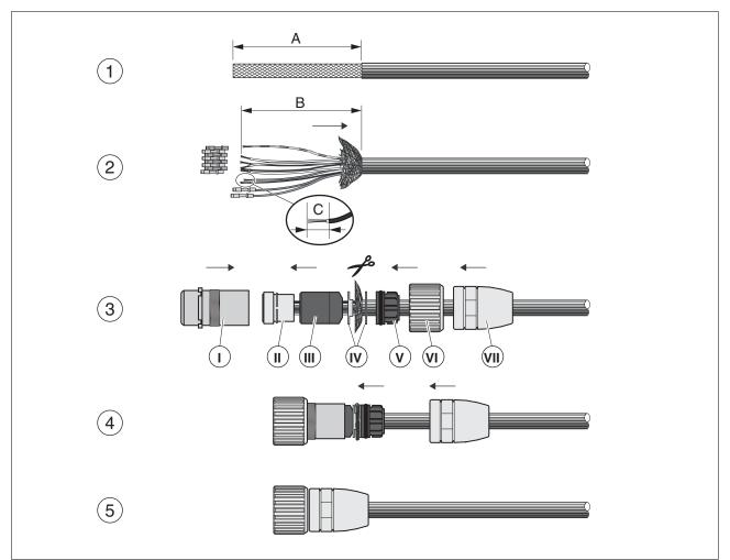
Figure 12: Assembling encoder cables with M23 encoder connector
