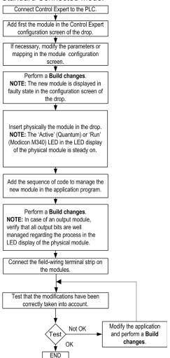
NOTE: One Ethernet RIO drop can have up to 4 modules added in one CCOTF transaction.
