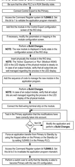
NOTE: One Ethernet RIO drop can have up to 4 modules added in one CCOTF transaction.
