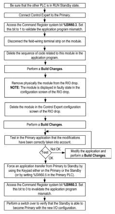
**NOTE:** One Ethernet RIO drop can have up to 4 modules deleted in one CCOTF transaction.
