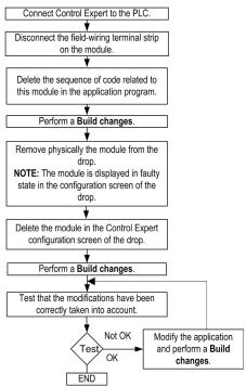
**NOTE:** One Ethernet RIO drop can have up to 4 modules deleted in one CCOTF transaction.
