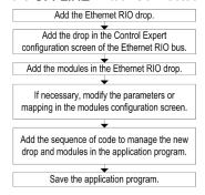
NOTE: A remote I/O drop contains 1 or 2 racks (linked with a backplane expander cable).
