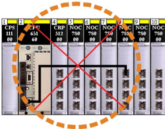
**Module Installation with 140CRP31200 Module Interlink**
