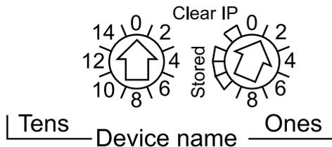
The values you set are applied during a power cycle. If you change the switch settings after the module has powered up, the Mod Status LED is activated and a mismatch message is logged in the module diagnostic.
