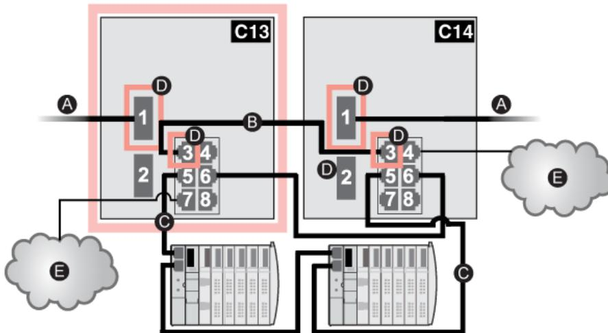
**C13** master DRS using a C13 predefined configuration file acting as the primary redundant connection between the main ring and the distributed I/O sub-ring
