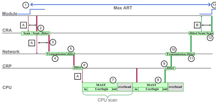
**NOTE:** Overhead in the previous illustration refers to the time period between the end of MAST processing (noted by the end of **out**) and the start of the next period (based on PLC MAST cycle time).
