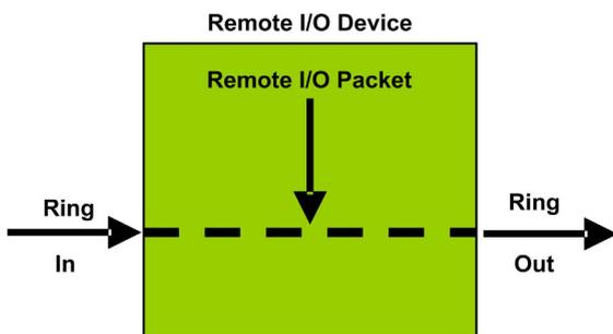
The remote I/O device handles remote I/O packets in the following sequence:
