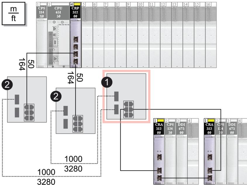
**Note:** The dashed line represents fiber cable, and the solid line represents copper wire.
