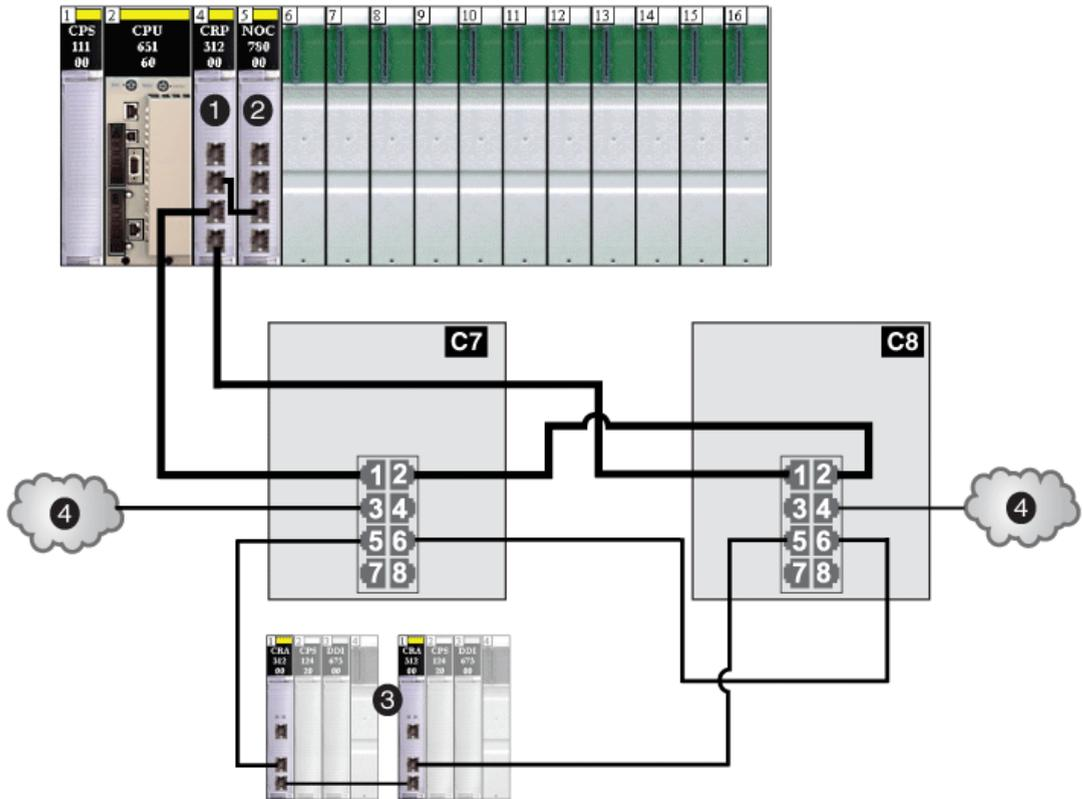
**C7** a DRS using the C7 predefined configuration file for a *master* copper remote I/O main ring with a remote I/O sub-ring and distributed I/O clouds
