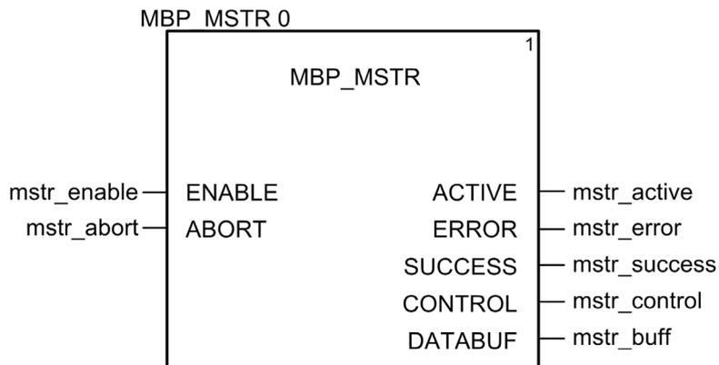
In the Control Expert application, write an MSTR block to send an EIP explicit message to the DRS that is managing the sub-ring. This EIP explicit message can be sent via the 140CRP31200 module or other communication module that is managing devices in the device network.
