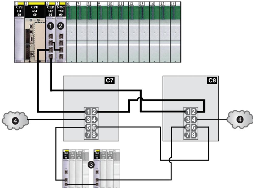
**C7** DRS using the C7 predefined configuration file for a *master* copper remote I/O main ring with a remote I/O sub-ring and distributed I/O clouds
