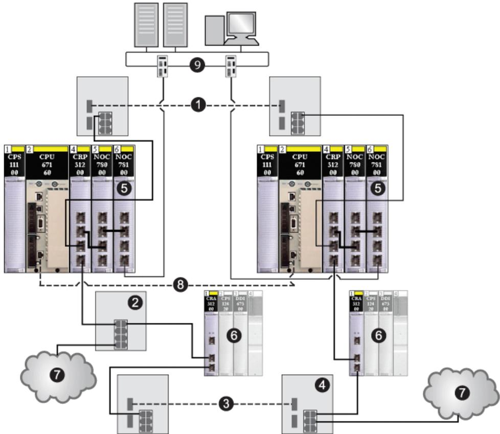
**NOTE** A DRS predefined configuration, C15, is available for the switches that support a fiber link between the primary and standby controllers.
