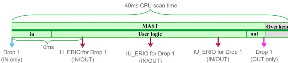
With the insertion and spacing of immediate update I/O blocks, the ART in the above example would be one-fourth of the original.
