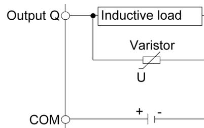
In applications where the inductive load is switched on and off frequently and/or rapidly, ensure that the continuous energy rating (J) of the varistor exceeds the peak load energy by 20% or more.
