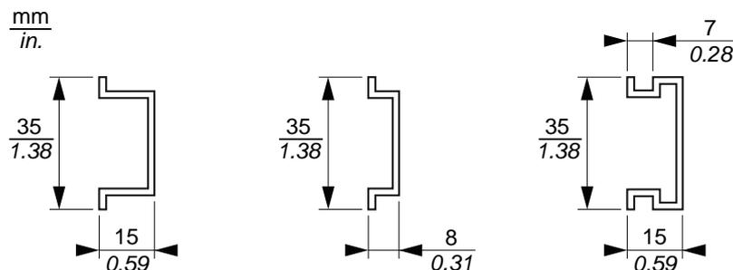
You can order a suitable DIN rail from Schneider Electric:
