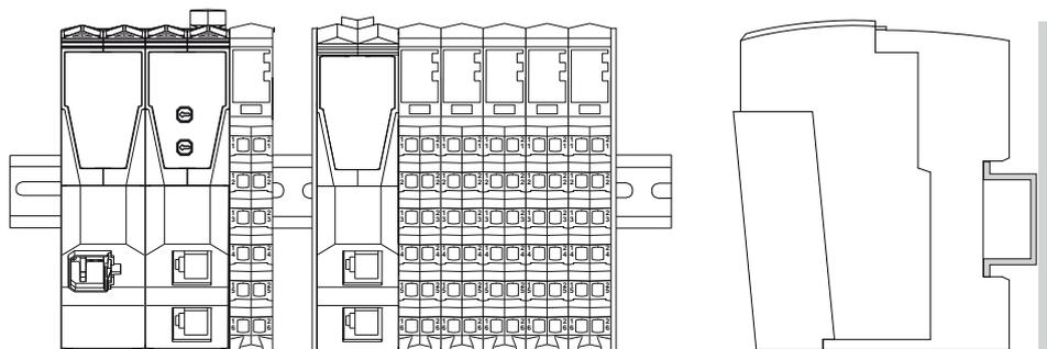
**NOTE:** The Safety Controller TM5CSLC100FS/TM5CSLC200FS or TM5CSLC300FS/TM5CSLC400FS can only be connected with the safety-related modules via the Sercos III Bus Interface TM5NS31. There is no electrical connection between Safety Controllers and the safety-related modules via the bus base.
