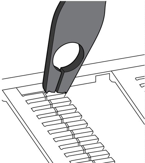
A line drawing of a terminal block with a row of slots. A labeling tool with a circular hole and two cutting edges is positioned over one of the slots, gripping a small tab protruding from it.                                                                                        |
