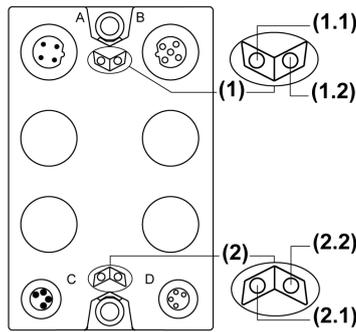
**(1)** TM7 power bus status LEDs, set of two LEDs: 1.1 (green) and 1.2 (green)
