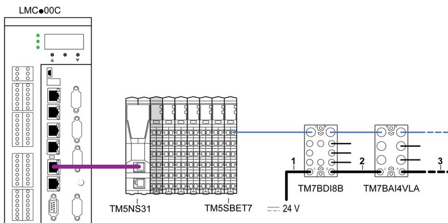
**1** Attachment IN cable: to connect an external power supply to a TM7 interface I/O block, a TM7 Power Distribution Block (PDB) or a TM7 I/O block.
