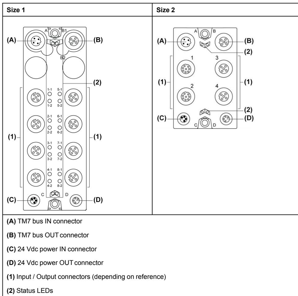
**NOTE:** For more information on the pinouts of these various connectors, see Modicon TM5/TM7 I/O Safety Modules Hardware Guide (see Modicon TM5/TM7, I/O Safety Modules, Hardware Guide).
