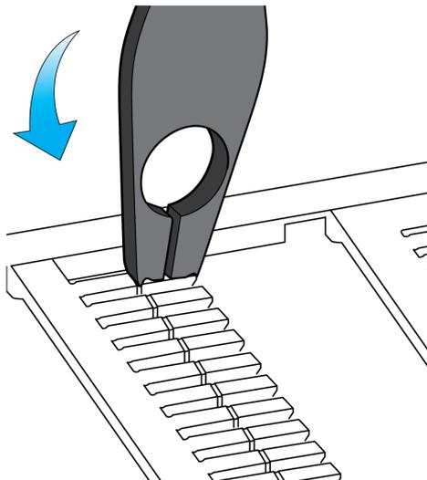
A line drawing of the terminal block and labeling tool from the previous step. A blue curved arrow points downwards from the tool's cutting edge, indicating the direction of pressure applied to separate the label tab.                                                              |
