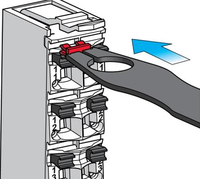
A perspective view of a terminal block with three rows of slots. The top row has a red label tab protruding from a slot. A labeling tool is positioned over the tab, and a blue arrow points to the right, indicating the direction to move the tool to center the tab over the slot. |
