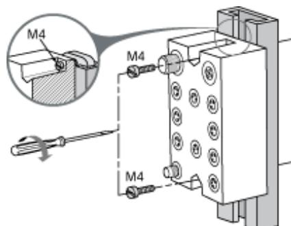
**NOTE:** Maximum torque to fasten the M4 screws is 0.6 N.m (5.3 lbf-in).
