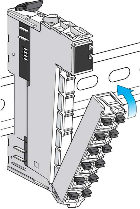
A technical illustration of an electronic module with a terminal block being rotated into place. A blue arrow indicates the upward rotation of the terminal block. The module has a vertical stack of components, and the terminal block is being aligned with a set of terminals on the right side. |
