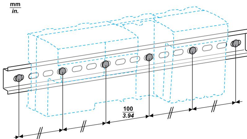
Low profile NSYSR200D DIN rail may be used with low profile mounting hardware such as flat head screws with countersunk mounting holes.
