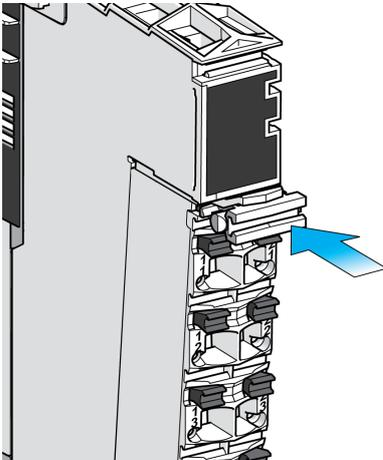
A technical illustration showing the terminal locking clip fully installed on the terminal block. A blue arrow points to the right, indicating the final position of the clip. The clip is now seated in the slot, securing the terminal block to the module.                                      |
