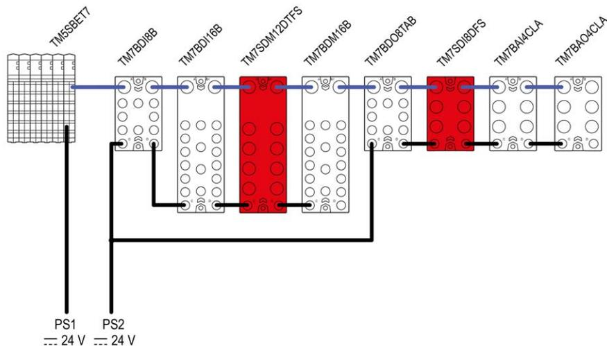
**PS1** External isolated main power supply, 24 Vdc
