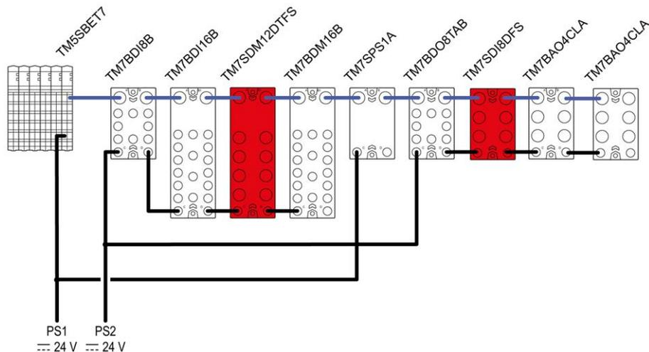
**PS1** External isolated main power supply, 24 Vdc
