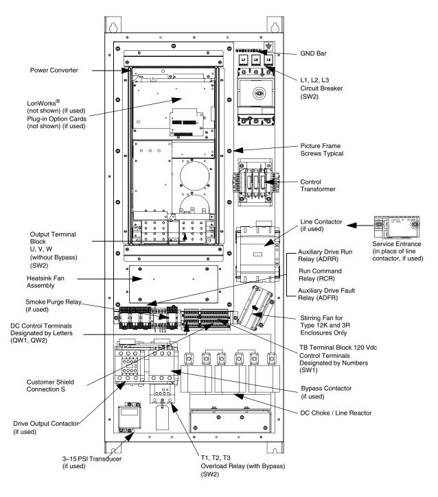
Figure 15 shows component identification and terminal strip locations for E-Flex drives 60–100 hp at 460 V and 30–50 hp at 208/230 V. Tables 22,
