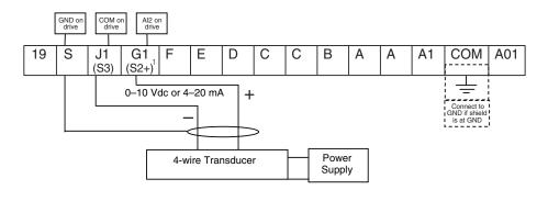
Terminal S2+ is not always wired to the drive and may need to be wired directly to the drive or as illustrated, a wire must be added from the drive to the terminal block.
