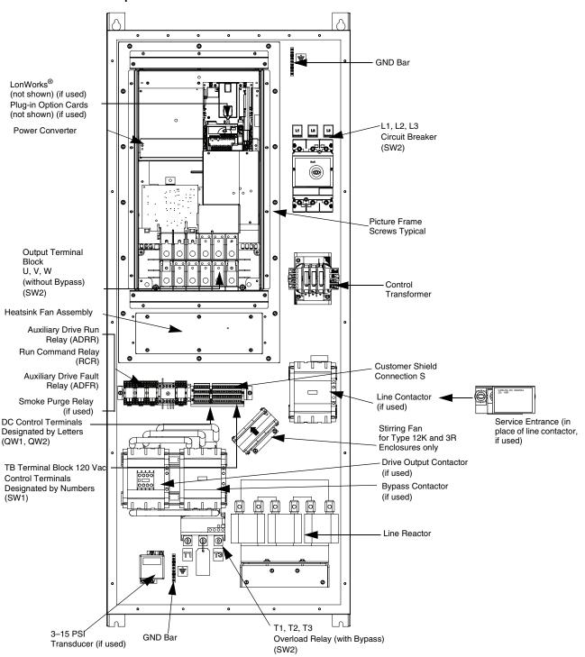
Figure 16: Typical Component Identification and Terminal Strip Locations Without Bypass for 60–100 hp @ 460 V and 30–50 hp @ 208/230 V
