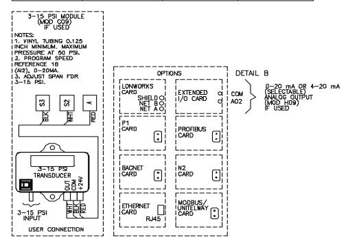
Figure 34: Power Circuit Y (With Bypass): Hand-Off-Comm, Start-Stop, and Speed Potentiometer (Drawing No. 80461-078-01)
