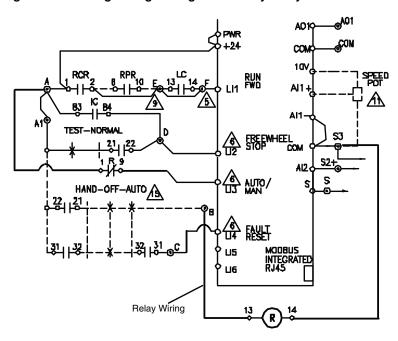
This method uses an auxiliary relay (+24 Vdc) energized by the HOA switch (if a spare relay is available at the installation site). Figure 26 illustrates the wiring changes described in this method. For example, a combination 8501NR45 (14-pin relay socket din rail mountable) and 8501RS14V20 (4-pole relay) may be used. See Section 6, "Power and Control Circuit Elementary Diagrams" on page 99 for complete wiring diagrams.
