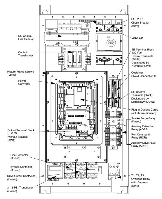
Figure 13 shows component identification and terminal strip locations for E-Flex drives 10-25 hp at 460 V and 7.5-10 hp at 208/230 V. Tables 22, 23, and 24 (pages 51-53) list wire size range and terminal torque requirements.
