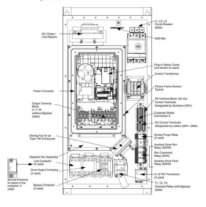
Figure 14 shows component identification and terminal strip locations for E-Flex drives 30–50 hp at 460 V and 15–25 hp at 208/230 V. Tables 22, 23, and 24 (pages 51–53) list wire size range and terminal torque requirements.
