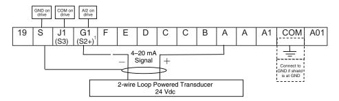
Figure 22: Separately Powered Transducer
