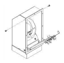
Figure 28: Removing Bracket Mounting Screws
