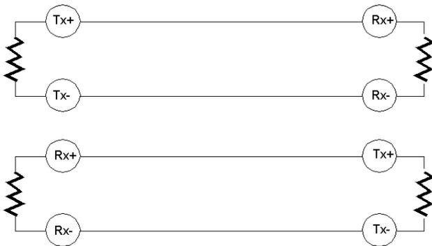
OR: 2 wire the terminals with 120  $\Omega$  only at each end of the network.
