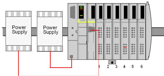
Here is a 24 V parallel power scheme for an Advantys STB island with a basic PDM:
