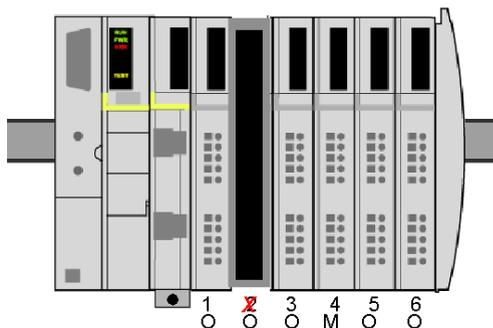
Again, the island will behave the same way as it would if all the modules were optional—all of the existing modules would continue to be operational. However, if you push the RST button while the module is removed the current configuration will be erased and only the module in location 1 will be operational.
