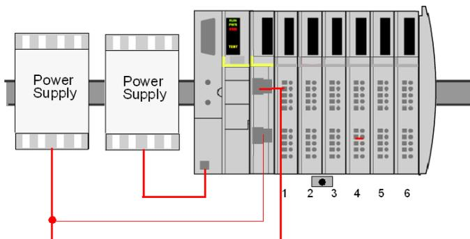
Here is a 24 V parallel power scheme for an Advantys STB island with a standard PDM:
