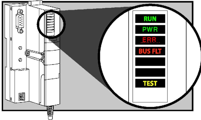
**NOTE:** The low-cost basic NIMs do not have a yellow TEST LED.
