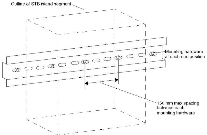
Low profile (7.5 mm deep) DIN mounting rail may be used with low profile mounting hardware such as flat head screws, with countersunk mounting holes.
