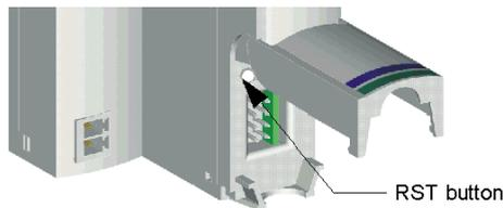
**NOTE:** Using the Advantys configuration software you can disable the reset button. In this situation pressing the reset button will not affect the existing configuration.
