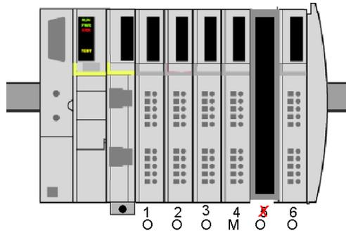
the island will behave the same way as it would if all the modules were optional—all of the existing modules would continue to be operational. Now, if the reset button is pushed your configuration will be erased and modules 1 through 4 will be default configured—all optional. If you power cycle instead of pushing the reset button, all the existing modules, except for the module in position 6, will be operational again and module 4 will continue to be configured as mandatory:
