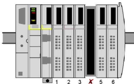
If you then place a new STB DDO 3230 output module in location 4, the NIM will recognize its device profile, configure it like the old module, and start supporting all six I/O modules the same as it did before the hot swap.
