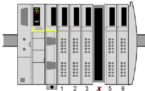
and then the RST button on the NIM is pushed, the modules in locations 1, 2 and 3 will remain operational, and the modules to the right of the empty location will not be detected.
