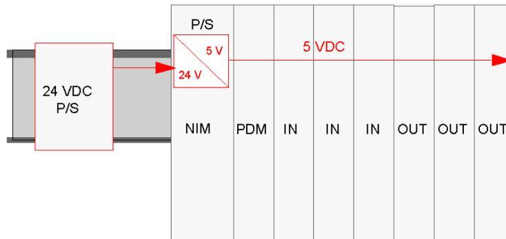
The maximum current draw from the I/O modules is limited to 1.2 A. If you place more I/O modules in the primary segment than the NIM's power supply can support (requiring more than 1.2 A of current), you may install an STB CPS 2111 auxiliary power supply to provide logic power to the additional I/O modules.
