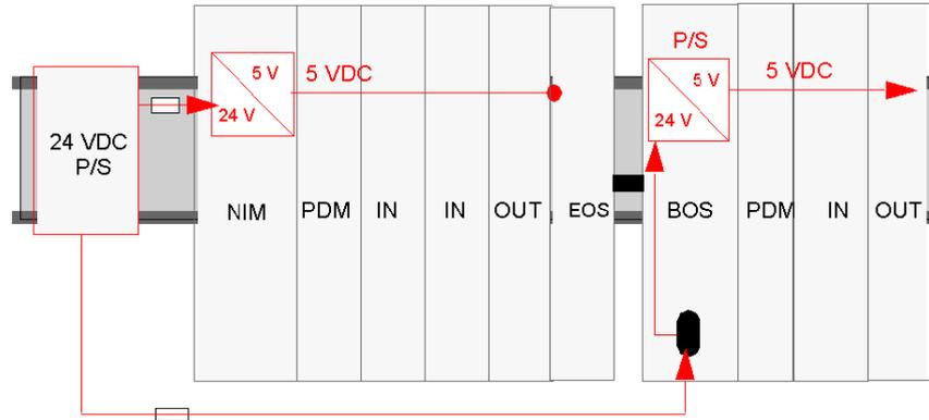
The external power supplies that you select to provide 24 VDC for logic power must have a low voltage limit of 19.2 VDC and a high voltage limit of 30 VDC.
