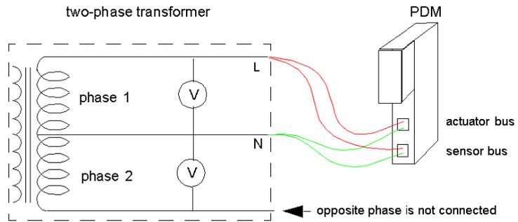
If the island segment contains a mixture of both 115 VAC and 230 VAC I/O modules, you must take care to install them in separate voltage groups and support the different voltages with separate STB PDT 2100 PDMs as is shown in the following illustration:
